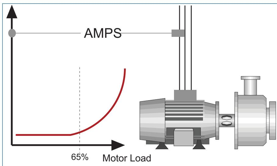
Figure 1. Motor Current vs. Load
